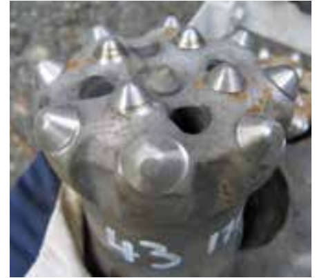
Norrtälje, Sweden. Secoroc Powerbit T45, 76 mm retrac, with HD Trubbnos buttons. The Trubbnos profile is re-created after grinding, keeping a wear flat area of about 10 %.
